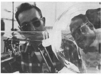
CAREFUL APPLICATION of the glassblower's art is required as Bert DuMars joins two glass pieces. The glass apparatus is a liquid nitrogen pump which will be mounted to an oil diffusion system.
